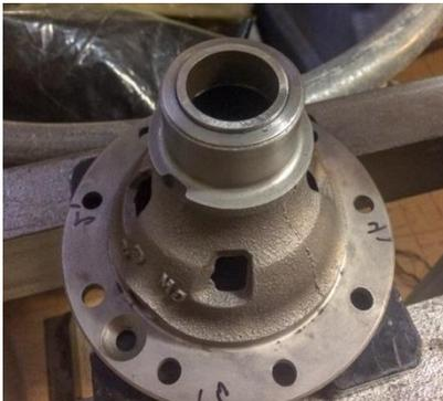
Step 4: Cut sleeves to length and press into the carrier halves. (Left)
