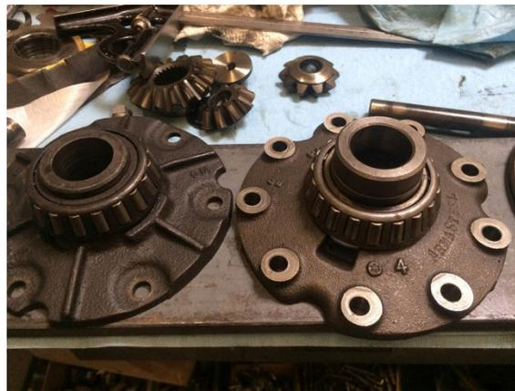
You can see the differences between the early and late differential components. The excess material above the bearings must be removed from the late parts so they'll fit in an early case.
