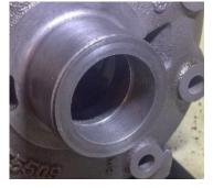
Step 2: We first need to bore out the ID the carrier halves to allow the insertion of a steel sleeve. What turned out to be the biggest hassle, was to get the part centered in my 4 jaw chuck! (Left)
