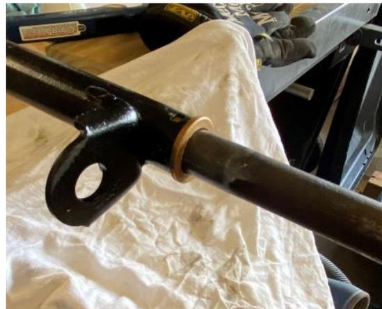
By August I had gathered or had on order most of the parts need and started cleaning/painting these parts. I tried Dave "Motohead" Watson's solution for the bronze bushings at the ends of the shift tube and found the "Flange Bearings on Amazon (The Hillman Group 58105 Flange Bearing, Bronze 3/4 X 7/8 X 1-1/8 X 3/4-Inch, 4-Pack). The outside diameter is perfect, the inside diameter does need to be opened up some to slide easily over the shift tube.
