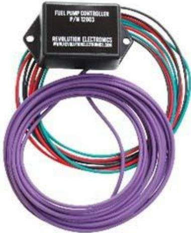
As long as you aren't off-roading it, I can't see how placing it tucked away by the tunnel would be an issue. If you can, go ahead and mount it under the dash. It doesn't make any noise. It gets a signal from your switched 12v and sends a 2 sec charge to the pump to prime the line at ignition. Then it automatically shuts off until it gets full 12v from the system. If it loses tach signal, it trips itself but will automatically re-set after sitting for a few min.
