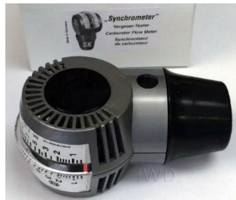
Snail” Type Air Flow Measuring Device
