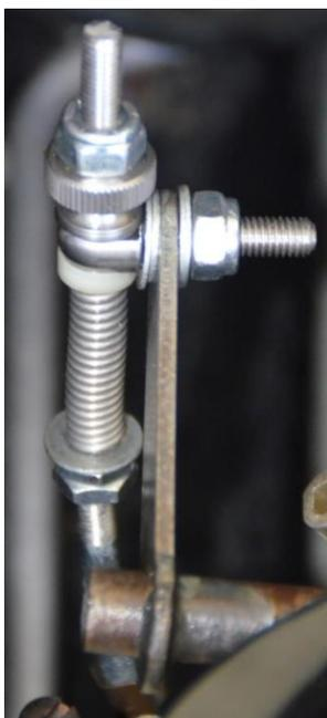
Basically, the lower clip is used but instead of using a threaded swivel and clip at the top, a smooth bore rod end is used that slides up and down as you adjust. To allow the movements yet hold position once adjusted, a compression spring is used to restrain the rod end. To make it "deluxe", you can even use a knurled adjusting nut (as shown in the photo). To allow movement at the pivot points, washers are used and are adjusted to not bind.
