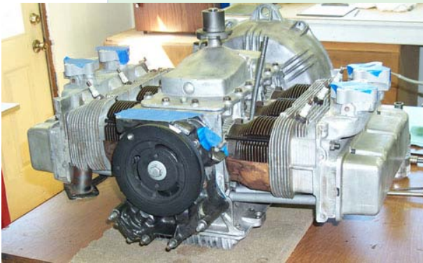
Gratuitous image of fast Corvair engine. Looks like a standard slow Corvair engine, but for slant exhausts and ultra-racy carb rotator adapters for the four ancient Rochesters...
