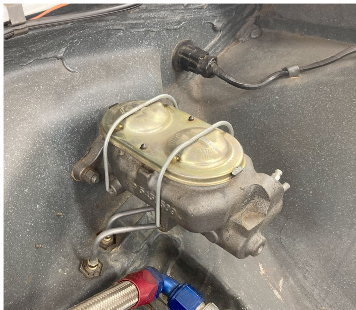
Yenko Stinger with dual MC. Two complete brake circuits versus one for the single MC. Image shows disk brake dual MC, will not match Clark's kit part in appearance.
