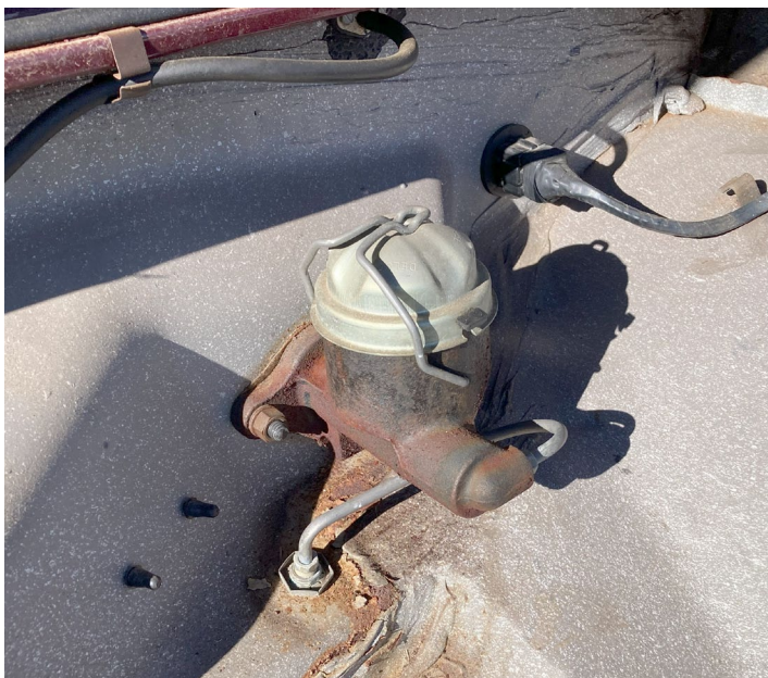
Single brake MC "Fruit Jar", typical on all Corvairs (except Yenko Stinger) through the 1966 model year.
