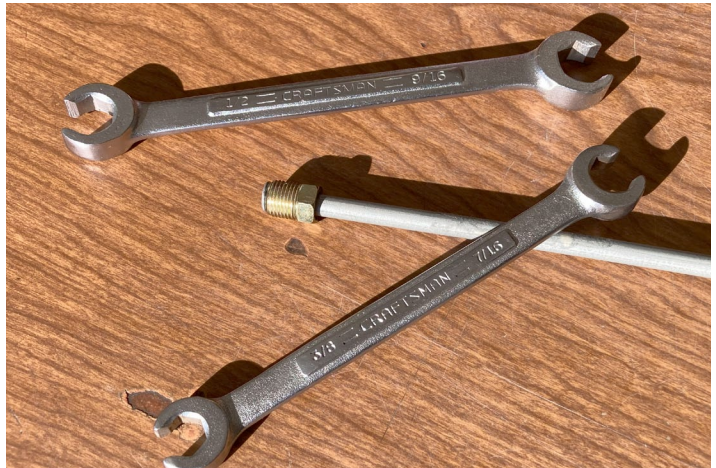
Flare nut wrenches, with male flare fitting. Note added grip flats.
