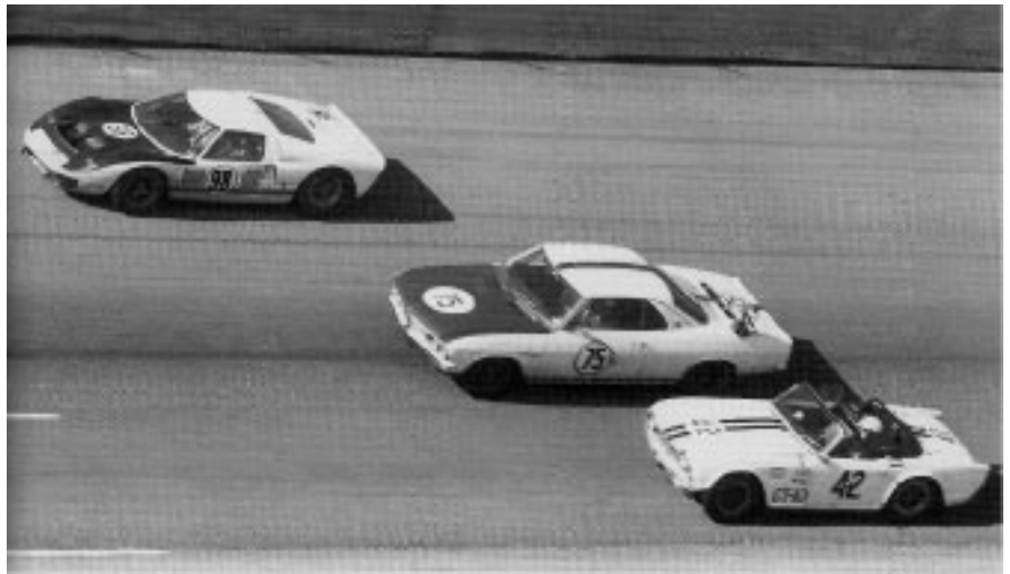
Stinger dicing with class competitor TR-4 on banking at Daytona, early in 1966. Note external oil cooler mounted on Stinger's left rear fender. It was relocated to a ducted front internal mount for subsequent events. And while it would be nice to believe the GT-40 was being passed, don't let that thought enter your mind, as its' passing differential speed was likely 40+ MPH.
