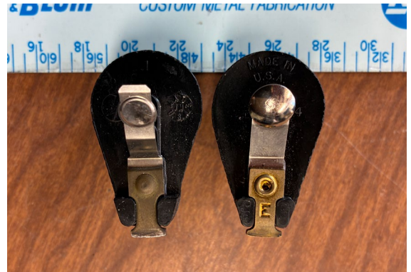
Two rotors sold as Corvair replacements. The one stamped with the emissions 'E' tip is shorter (they vary from 1/32" to 1/16" less), creating a wider gap to the cap contact terminal. E rotors are used with amplified ignition systems, and are NOT a good choice for Corvairs with standard point distributors.
