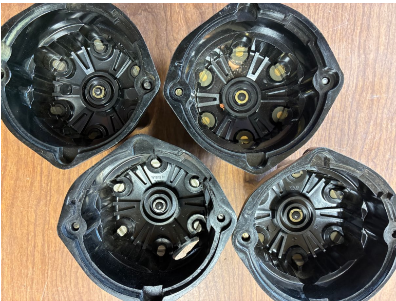
Four 'Corvair' distributor caps, identical from the outside, but each with different terminal materials and/or machining configurations. Avoid aluminum (lower left cap); copper (as in upper right cap) is the preferred material. Notch machining varies by supplier machine set up. Again, amplified ignition helps overcome manufacturing variance.
